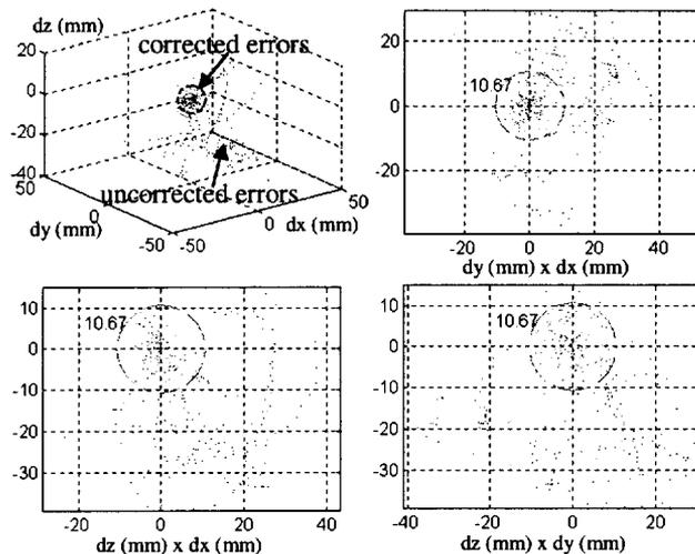
Figure 6 - Measured and Residual Errors After Compensation
