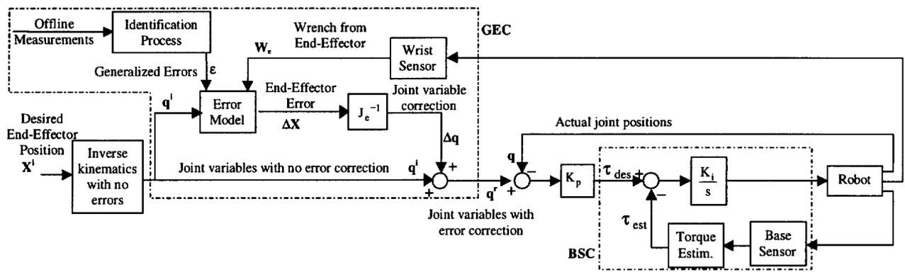
Figure 2 - Base Sensor Control and Error Compensation Scheme
