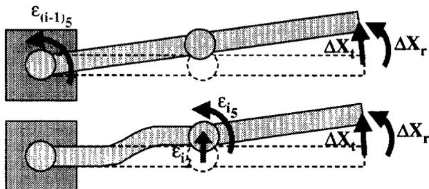
**Figure 4 – Error Combinations Resulting in Same End-Effector Errors**
