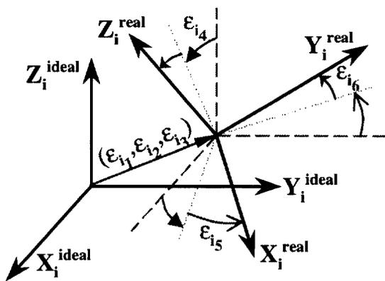
Figure 2 – Definition of the Translational and Rotational Generalized Errors for  $i^{th}$  Link
