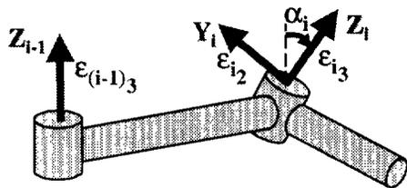
**Figure 3 – Linear Combination of Translational Generalized Errors**
