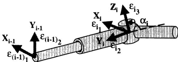
**Figure 5 – Linear Combinations of Generalized Errors in Prismatic Joints**
