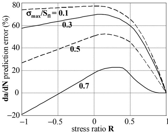
Figure 2. Non-conservative  $da/dN$  prediction errors for *plane strain* calculations based on *plane stress* data, according to Newman's closure function.
