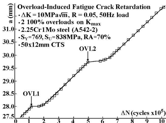
Figure 1. Fatigue crack growth retardation induced by tensile overloads [3].
