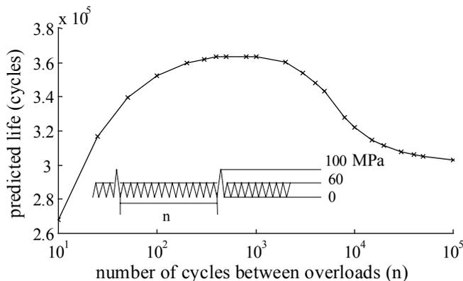
Figure 4. Generalized Wheeler life predictions for several simulated overload frequencies.
