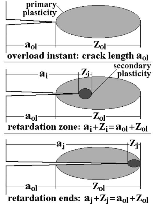
Figure 3. Yield zone crack growth retardation region used by Wheeler and by Willenborg.
