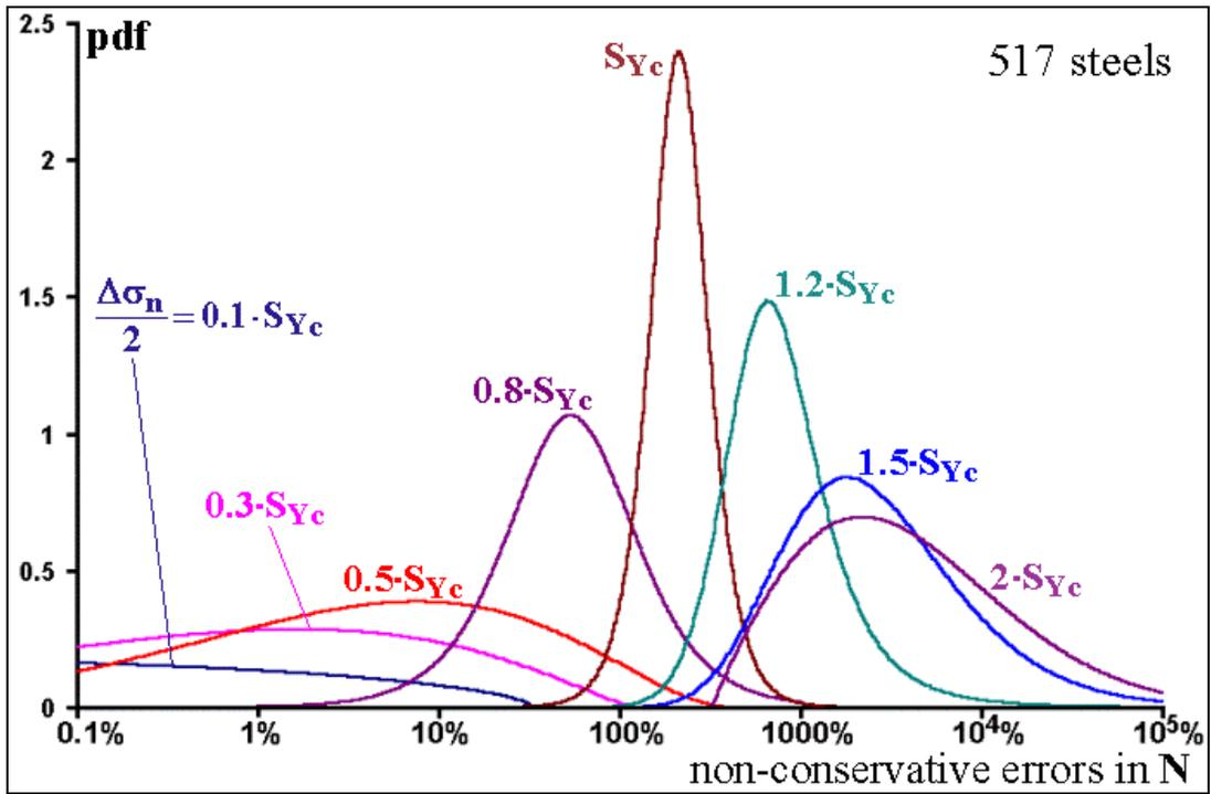
FIGURE 3 Statistics of the non-conservative errors in lives predicted by the classical Neuber approach, for several nominal stress levels (517 steels,  $K_t = 3$ ).
