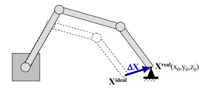
Figure 1. Real and Ideal Positions of a Manipulator End-Effector
