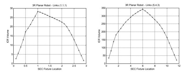
Figure 2. ICR Volume as a Function of the Fixture Location for Link Lengths (1, 1, 1) and (5, 4, 3)
