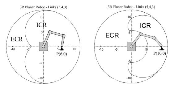
Figure 3. Extrapolated and Interpolated Compensation Regions for an SEC Fixture at (6,0) or (10,0)
