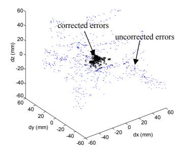
Figure 5. Measured and Residual Errors After Compensation
