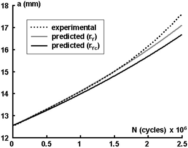
Figure 3: Comparison between crack growth measurements and  $\epsilon N$ -based predictions
