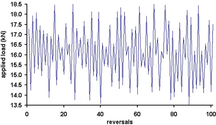
Figure 2: Load block applied to the CTS
