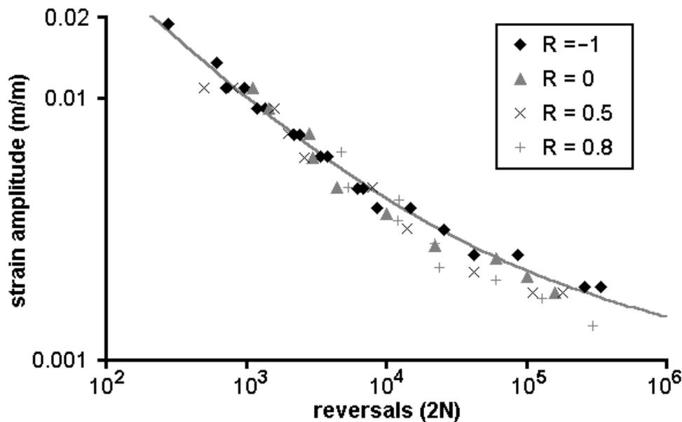
Figure 1: Measured and fitted strain-life data for the API 5L X52 steel
