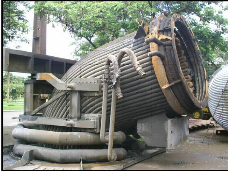
Fig.1: A steel furnace hood, made by welding properly curved low-carbon steel tubes.
