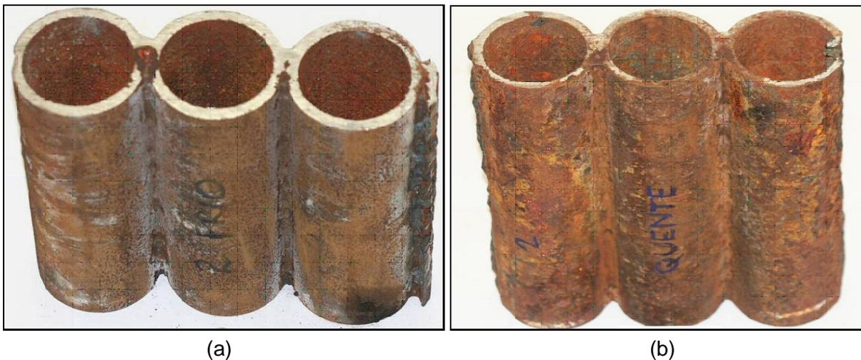
Fig.2: Sample of a cracked hood tubular wall (a) cold part, which faced the atmosphere, and (b) hot part, which faced the furnace output gases. Note the corrosion with several pits on this hot wall surface and also on the water cooled wall surfaces, inside the A106 steel tubes.
