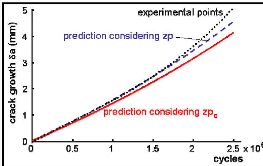
Fig. 9. Comparison between crack growth measurements and  $\epsilon N$ -based predictions for the variable amplitude load presented in Fig. 8 (API-5L-X52 steel).
