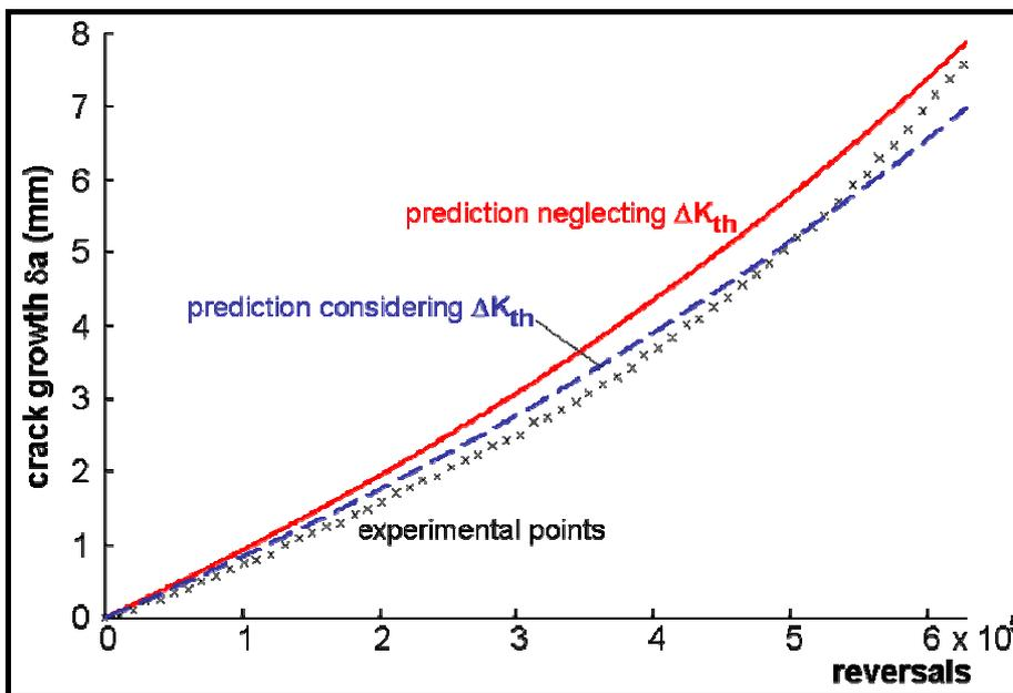
Fig. 11. Comparison between crack growth measurements and  $\epsilon N$ -based predictions for the variable amplitude load presented in Fig. 10 (SAE 1020 steel).
