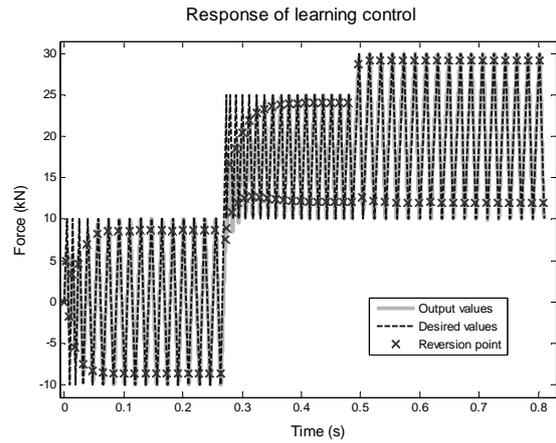
Figure 6. Learning control responses for a variable amplitude input.
