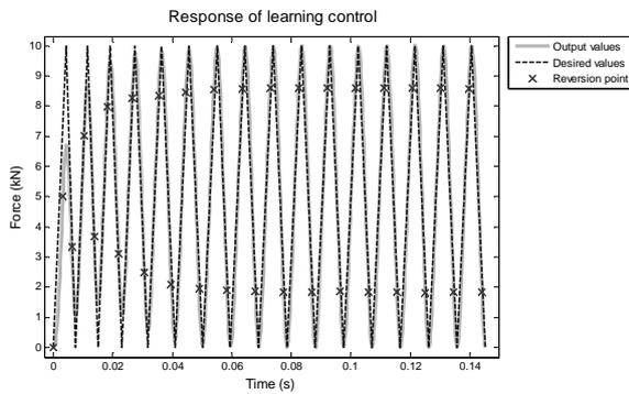
Figure 4. Learning control responses for a constant amplitude history from 0 to 10kN
