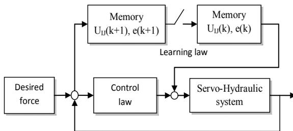
Figure 1. Block diagram of the learning control
