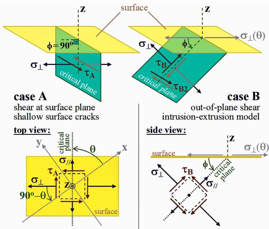
Figure 1: Case A and Case B cracks.
