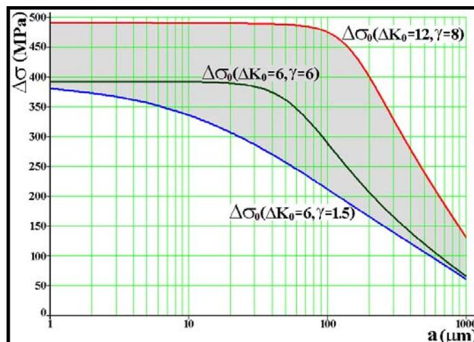
Figure 3: Typical steel threshold  $6 < \Delta K_0 < 12 \text{MPa}\sqrt{\text{m}}$  and  $\gamma$  exponent  $1.5 < \gamma < 8$  ranges influence in the largest mode I stress ranges  $\Delta\sigma_0$  tolerated by the  $w = 3.4 \text{mm}$  strip, as a function of the 1D superficial crack size  $a$ .
