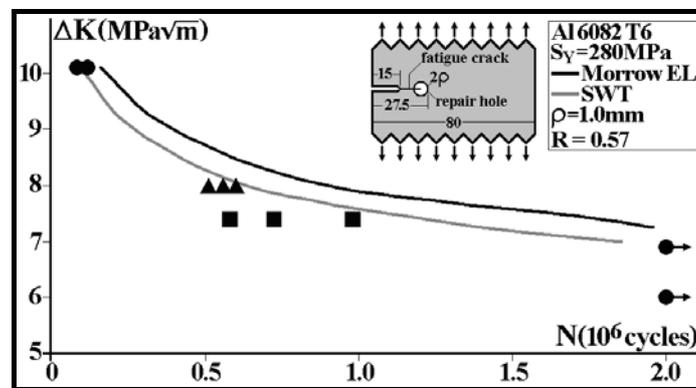
Figure 1: Predicted and measured crack re-initiation lives after introducing stop-holes with radii  $\rho = 1.0mm$  at the tip of the previous crack, using the properly calculated  $K_f$  of the resulting elongated slit (instead of its  $K_t$ ) and  $\varepsilon N$  procedures.
