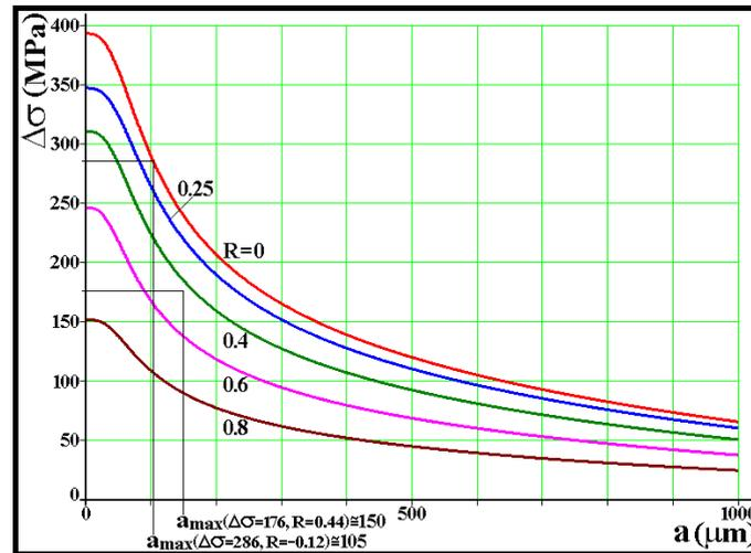
Figure 2: Surface crack of size  $a$  effect in the largest stress range  $\Delta\sigma_R(a)$  tolerable by a strip of width  $w = 3.4 \text{mm}$  loaded in mode I, for various  $R$ -ratios (supposing  $\Delta K_0 = 6 \text{MPa}\sqrt{\text{m}}$  and  $\gamma = 6$ , thus  $a_0 = 59$  and  $a_{0.8} = 55 \mu\text{m}$ ).
