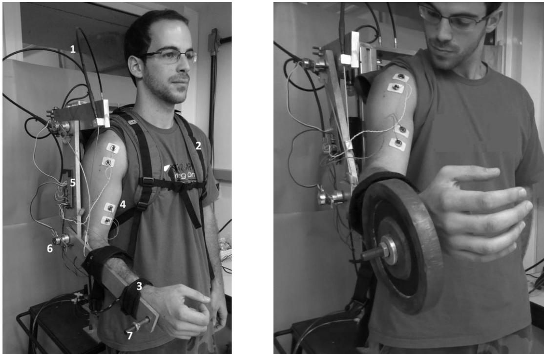
Figure 8. The exoskeleton system (left); and a trial with a 7 lb (3.2kg) payload (right)
