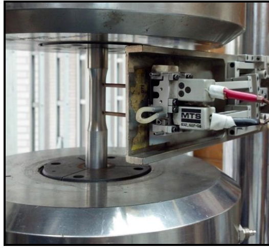
Fig. 6: Tubular tension-torsion specimen mounted in an MTS tension-torsion machine, showing the axial/torsional extensometer.
