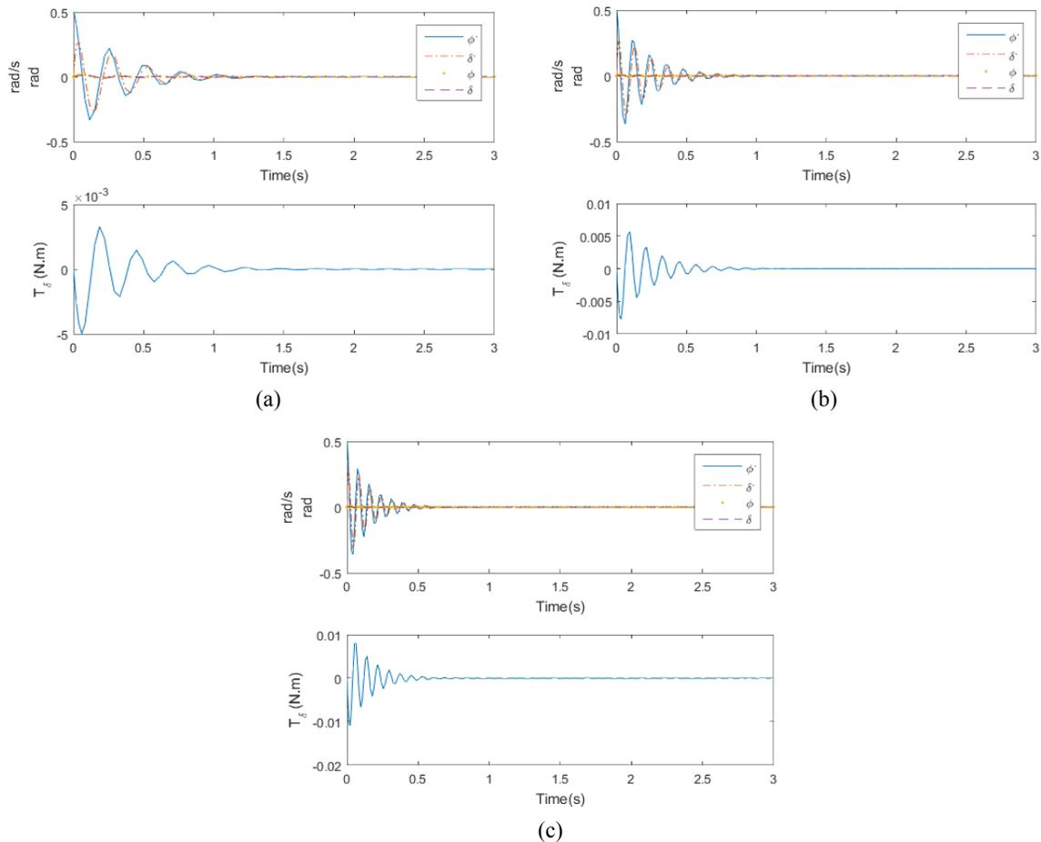
Figure 4 – Simulation to stabilization state feedback at: (a) 5 m/s; (b) 10 m/s; (c) 15 m/s.
