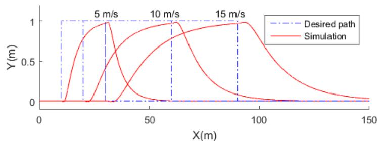
Figure 6 – Comparison between trajectory control at: (a) 5 m/s; (b) 10 m/s; (c) 15 m/s.
