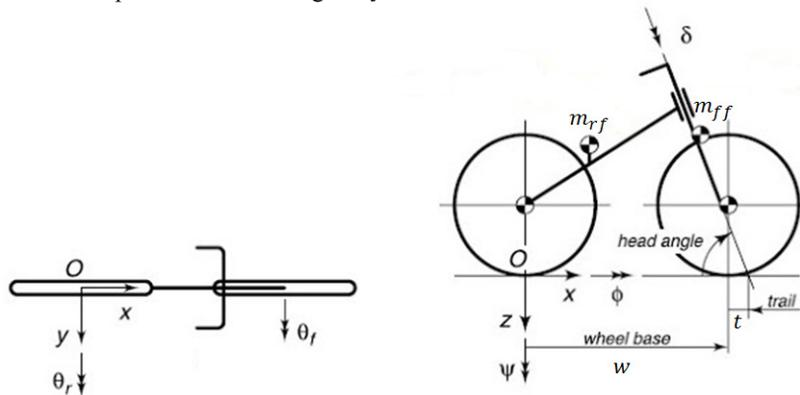
Figure 1 – Schematic of motorcycle's main parameters.
