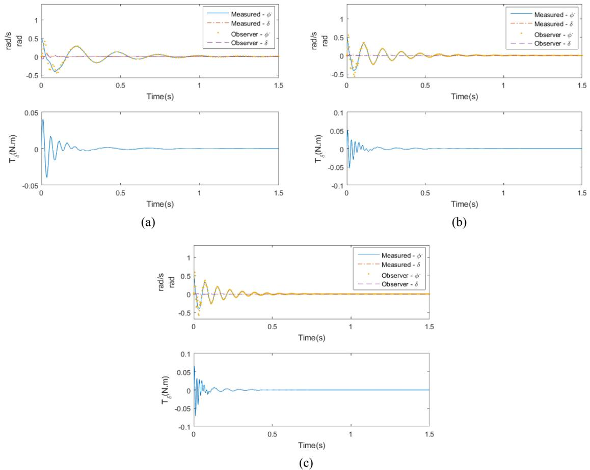
**Figure 5 – Simulation to stabilization state feedback with observer at: (a) 5 m/s; (b) 10 m/s (c)15 m/s.**
