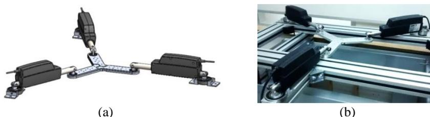
Figure 1 – CAD model of the planar mechanism (a) and the built platform (b).
