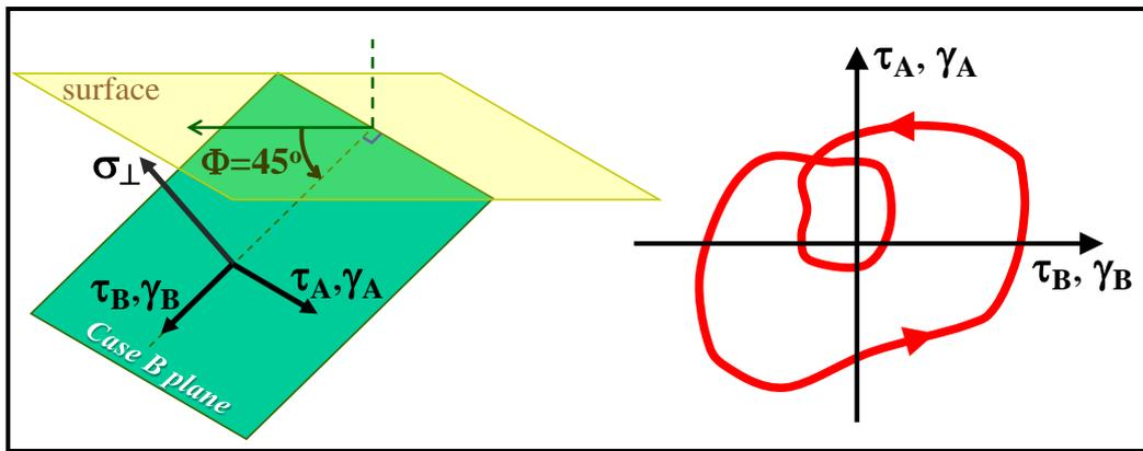
**Fig. 2:** NP shear strain path  $\gamma_B \times \gamma_A$  (or shear stress path  $\tau_B \times \tau_A$ ) acting on candidate planes at  $45^\circ$  from a free surface, for a general loading history.
