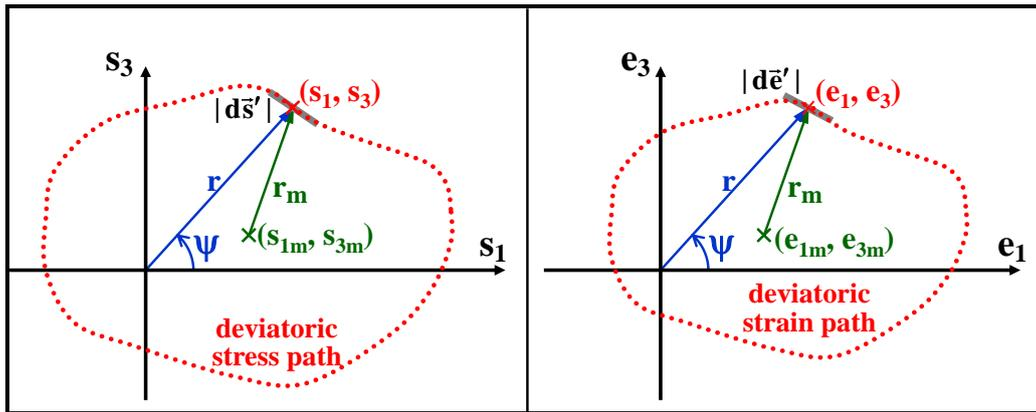
**Fig. 1:** Stress path of a 2D tension-torsion load history in a deviatoric stress diagram (left) and its corresponding strain path in a deviatoric strain diagram (right), both assumed as homogeneous wires with unit mass.
