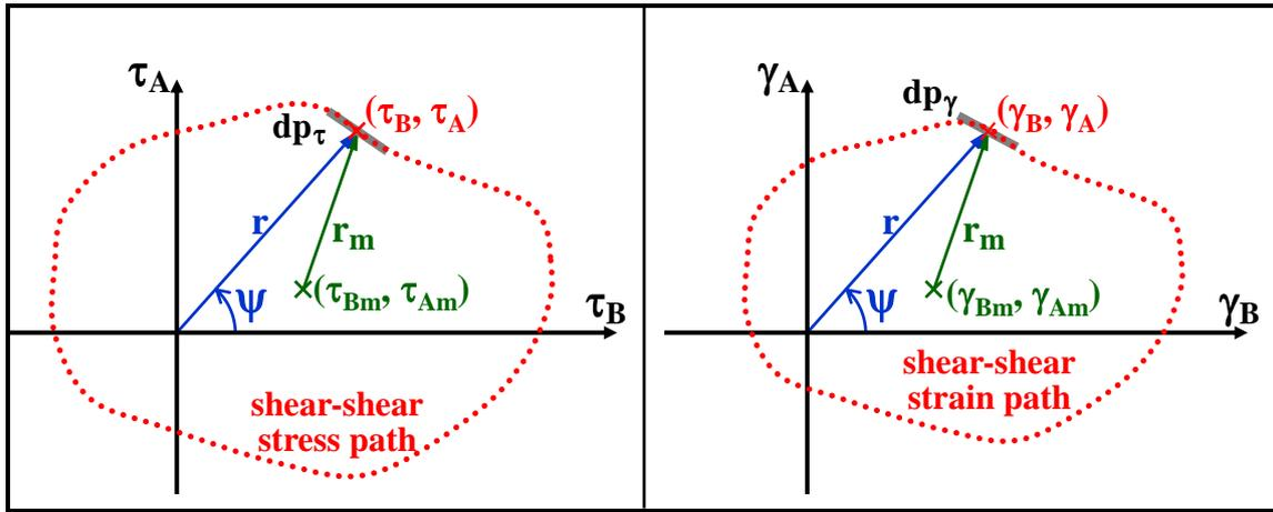
**Fig. 3:** Stress path of a 2D shear-shear history on a candidate plane (left) and corresponding strain path (right), both assumed as homogeneous wires with unit mass.
