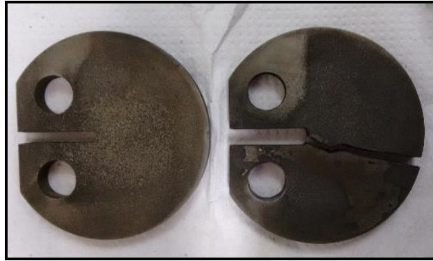
Figure 5: LE specimens after 30 days under EAC in aqueous hydrogen sulfide environment.
