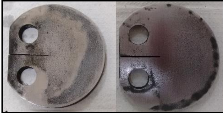
Figure 8: EP specimens after 30 days under EAC in aqueous sulfide environment.
