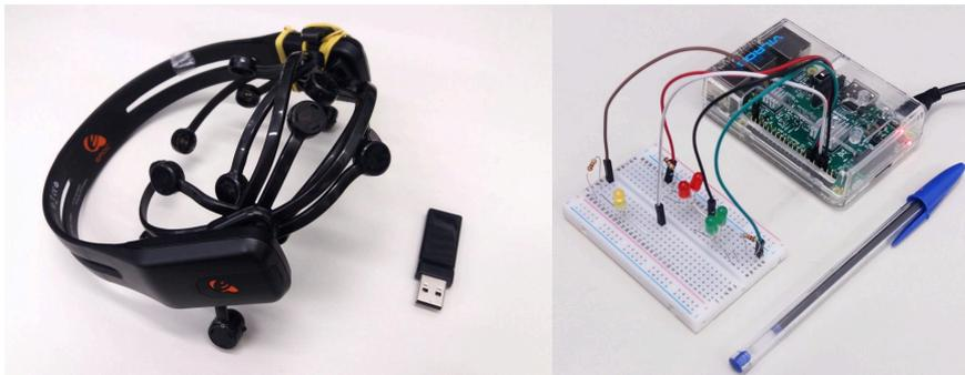
Figure 2. Emotiv Epoc Headset, the EEG equipment, and the Bluetooth dongle (left), and Raspberry Pi connected to the output circuit (right).
