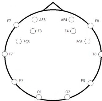
**Figure 6. Electrodes positioning in Emotiv, according to the 10-20 extended system.**
