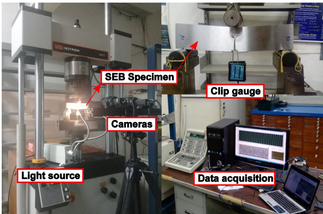
Figure 8. Experimental setup used to measure the J-R curves and displacement fields on the specimen surface using the VIC-3D system.
