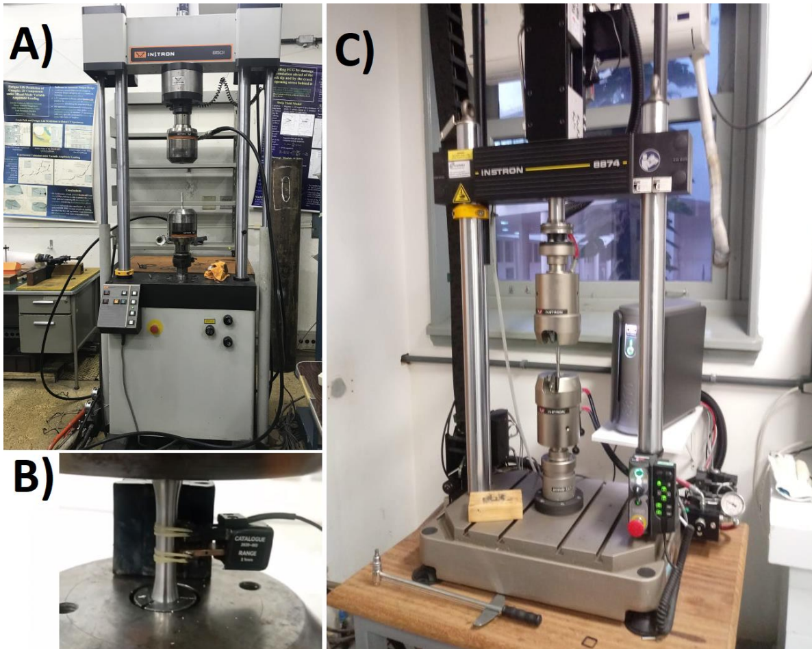
Figure 2. A) Instron 8501 Servohydraulic Fatigue Testing System; B) Instron 2630-100 Series Clip-on Extensometer; C) Instron 8874 Biaxial Servohydraulic Fatigue Testing System.
