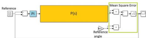
Fig. 6: Figure showing the block diagram with a fixed angle at closed loop with PI controller
