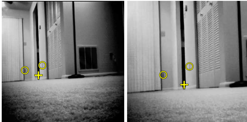
Fig. 4. Robot view tracking to child node (+) with the aid of fiducials (o)
