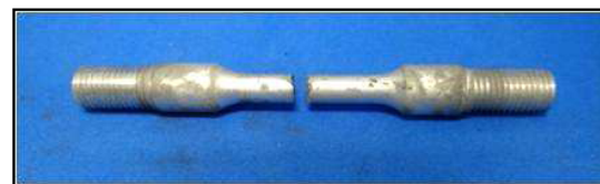
Fig. 18 Initially smooth test specimen with 6.35 mm diameter, used for measuring S_{SCC} , the resistance to crack initiation under SCC, according to ASTM F1624 and ISO 7539 standards.
