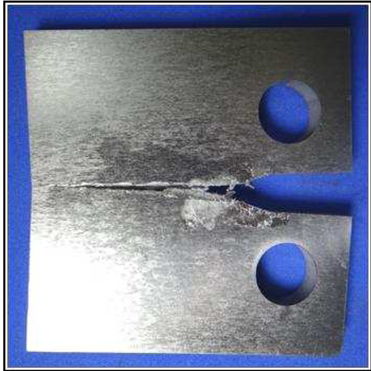
Fig. 19 C(T) specimen with w = 60 mm used for measuring K_{ISCC} , the resistance to crack propagation under SCC, according to ASTM E1681, ASTM F1624, and ISO 7539 procedures.
