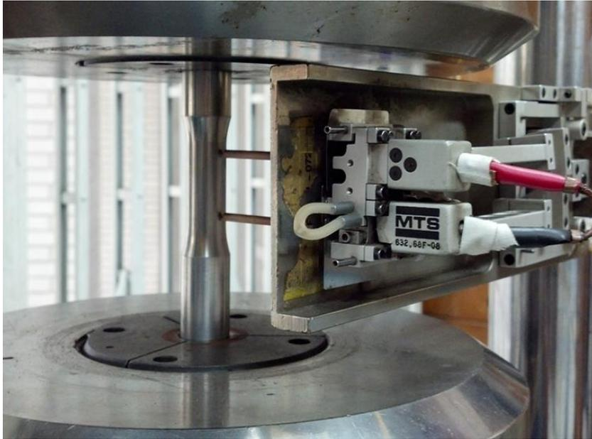
Fig. 3: Tension-torsion testing machine and extensometer.
