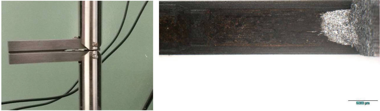
Figure 12: DCB specimen loaded by an imposed displacement in a servo electromechanical testing machine at equilibrium wedge-load (left), before it was immersed in the aggressive solution, and its fracture surface after it was broken in liquid nitrogen (right).
