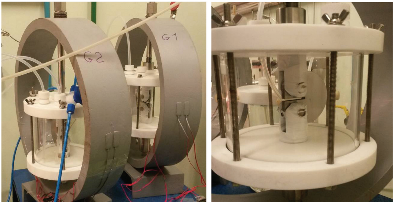
Figure 14: EAC tests of the notched 4140 steel DC(T)-like specimens used to verify the tolerance to short cracks under HE conditions predicted by the model proposed here (right), immersed in the aggressive solution and assembled in proof rings (left), and a front view of one of them.
