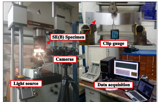
Fig. 12. Experimental setup used to measure the J - R curves and displacement fields on the specimen surface using the VIC-3D system.
