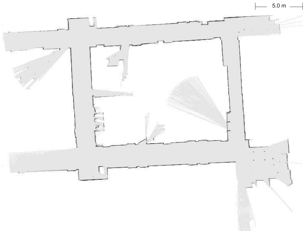
Figure 5.30: 2D grid map of "D-wing" experiment, acquired with DP-SLAM using the proposed motion model.
