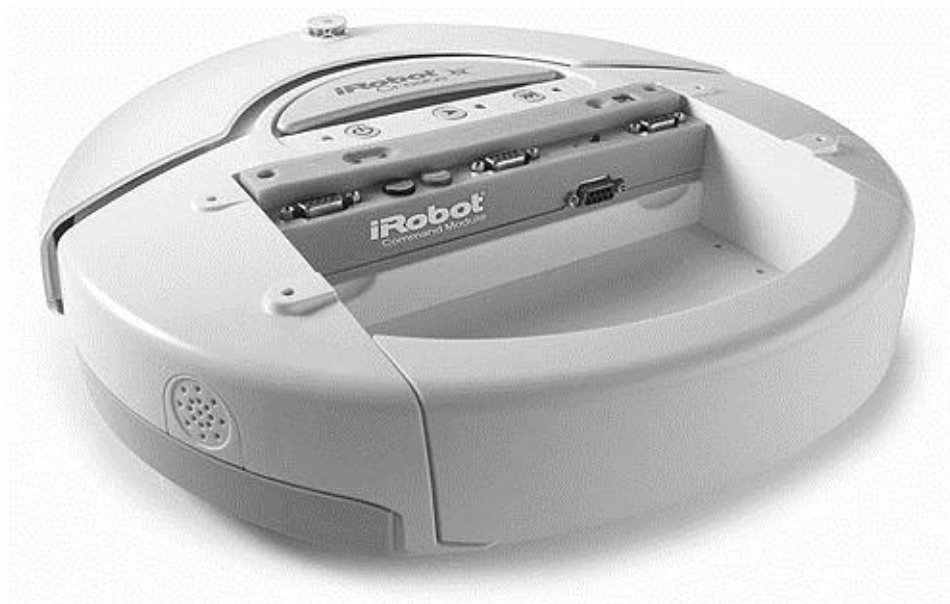
Figure 2: iRobot Create hardware with the iRobot Control Module .
