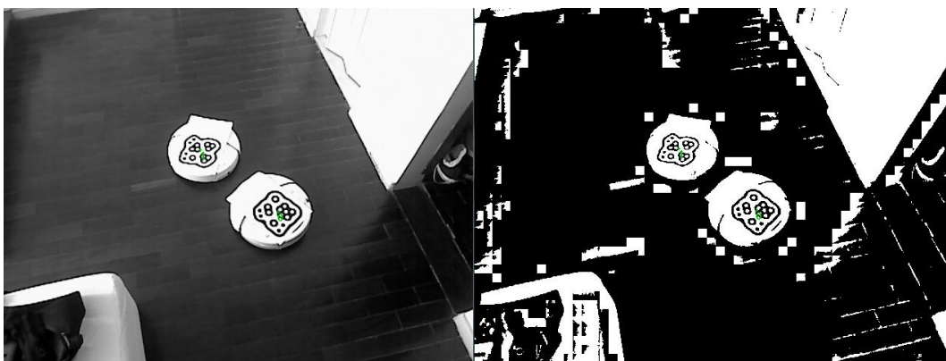
Figure 17: Raw greyscale image and the binary image by the Bernsen's binarisation method.
