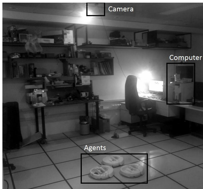
Figure 11: Real experimental setup with main components highlighted
