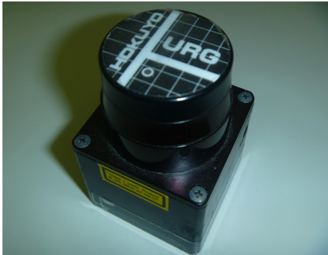
Figura 61: Laser Range Finder (LRF), Hokuyo URG 04LX-UG01.
