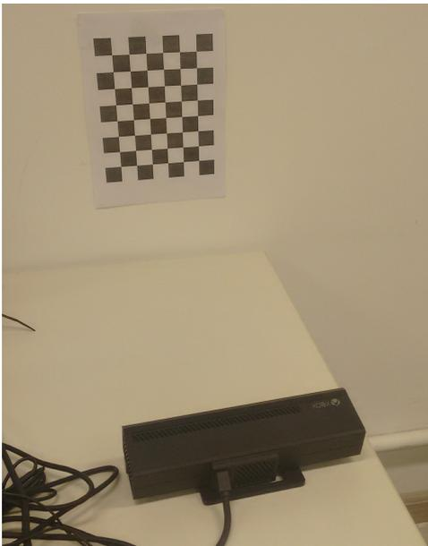
Figure 4.4: Kinect Calibration
