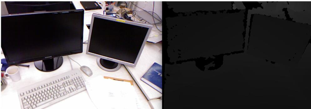
Figure 4.10: Registered color and depth frames
