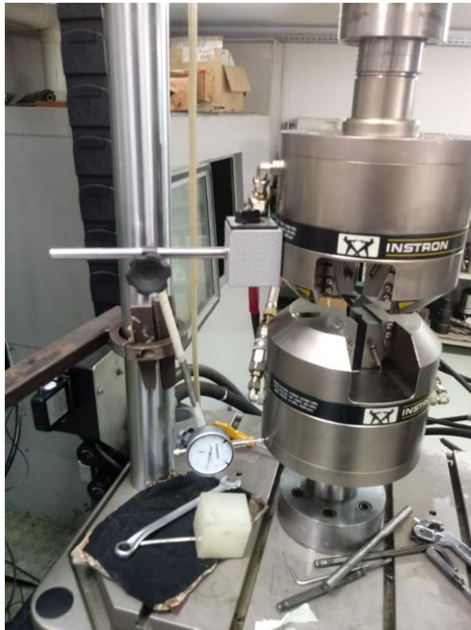
Figure 3.10: Example of an assembly for the Dial Indicator Method.
