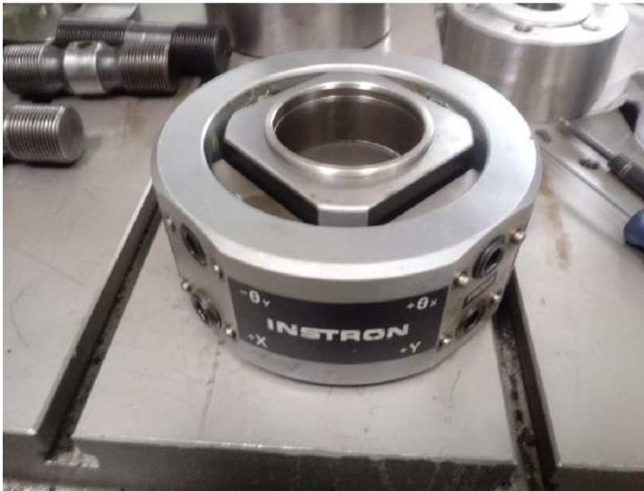
Figure 3.13: Instron Alignment Fixture Model 8000-073 (photo and schematic [15]).
