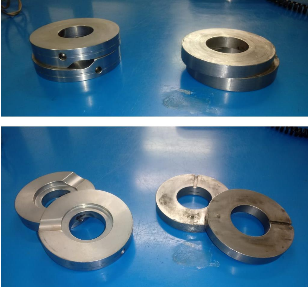
Figure 3.5: Two examples of pre-load washers. Helical pair on the left, inclined pair on the right.
