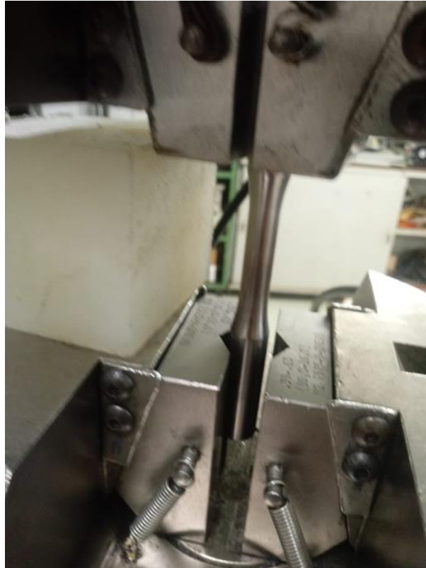
Figure 3.9: Example of a considerably misaligned assembly. The specimen should be within the same distance from each jaw face.
