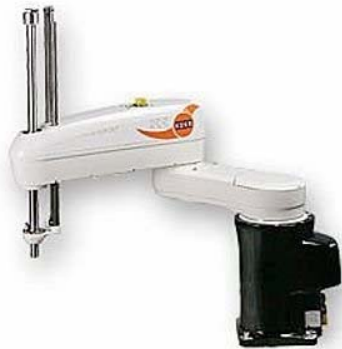
“SCARA Arm” (1979 - Sankyo and IBM), Selective Compliance Assembly Robot Arm
