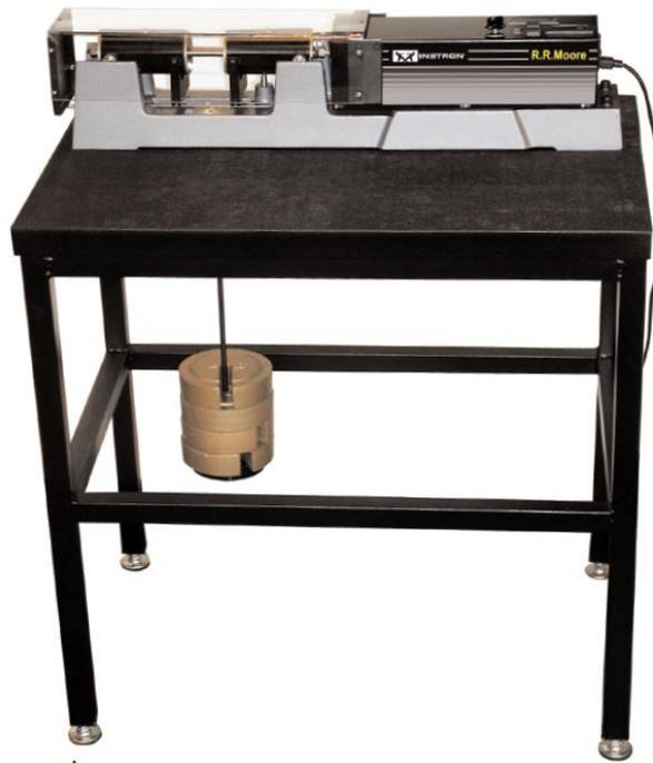
▲ R. R. Moore rotating beam fatigue testing system
